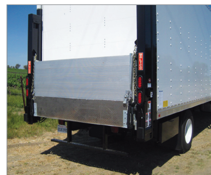
WDV Series Gate in stowed position offers simplicity and reduced maintenance
