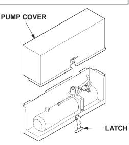
REMOVING / REINSTALLING PUMP COVER FIG. 9-1
